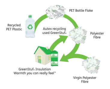
"The thermal bonding process allows GreenStuf® insulation to be further recycled and used again.
